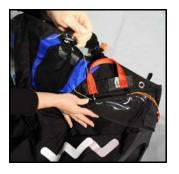
Push the metal pins on the handle into the elastic loops and under the transparent cover. It is essential to remove the cords after this operation. The cords should be pulled out slowly in order not to damage the elastic loops by excessive friction. Lastly, the handle should be positioned under the elastic cover.
