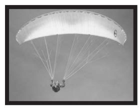
The **SYNCRO** is a **DHV** 2-3 glider that offers total security, along with beautiful handling & incredible performance. The performance is very high due to a well-defined structure with 69 cells, with an internal structure comprised of diagonals of different types, depending on the width of the cell and an optimized line layout to reduce the overall number of lines.
