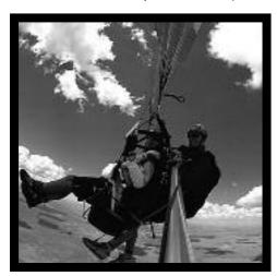
If your flying weight is above the stipulated weight range, this will result in a higher minimum speed and faster landing speed and the stall speed of the glider will also be higher. If the glider suffers a collapse, or leaves normal flight configuration, the resulting behaviour will be more rapid and violent. As well as this, your sink rate will be higher and you will find it harder to stay up in light lift.
